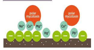
natural clinoptilolite surface (negative surface is caused by substitution of Si<sup>4+</sup> with Al<sup>3+</sup> or Fe<sup>3+</sup>)
